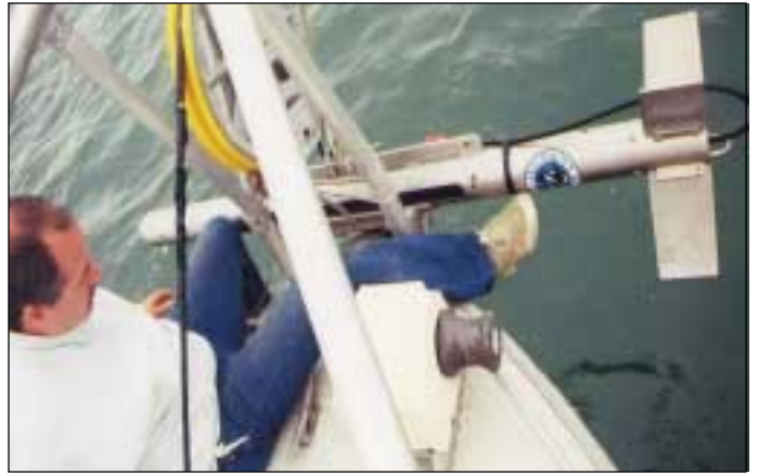
The torpedo-shaped “tow fish” sends out a sonar signal that allows researchers to see abandoned fishing gear beneath the water’s surface. Photo: J. Shaw
